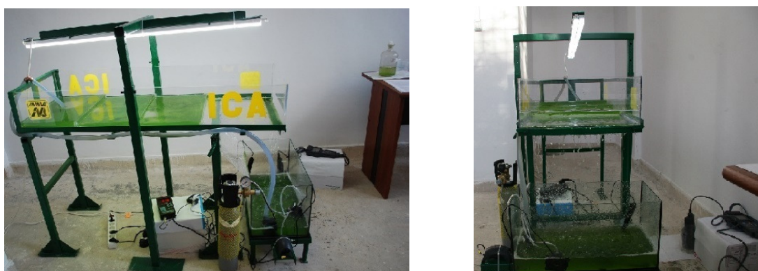
Fig. 3. Installation for algae cultivation in open system, cascade type during experiments
